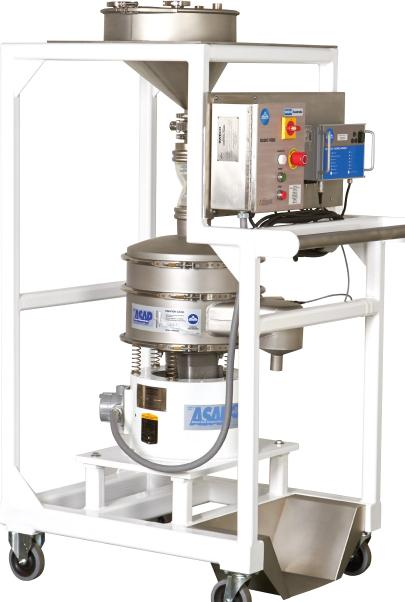
SWECO, the world leader in separation technology, introduces the 3D Metal Printer (3dMP) Screener System. This innovative design collects, screens, and rebottles reclaimed metal powder from 3D metal printers. The 3dMP Screener System is totally integrated, eliminating multiple operations and any material handling. The system is set up to feed in the used metal powder with agglomerates and discharge screened metal powder ready to be reused or mixed with virgin material.
